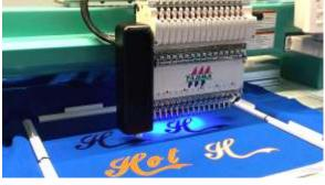
Thermal Cutting Device (TCD) for synthetic fabrics, that works in combination with the embroidery machine
